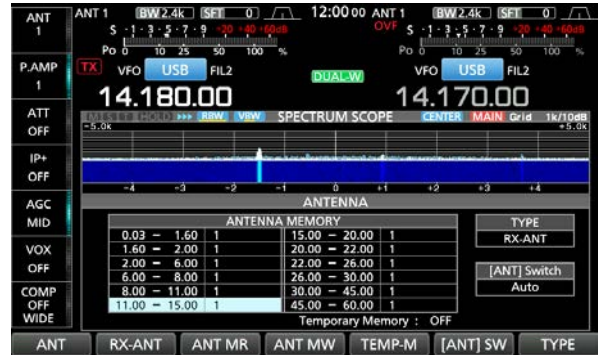
Example: Displaying the Mini scope screen while the ANTENNA screen is displayed.
